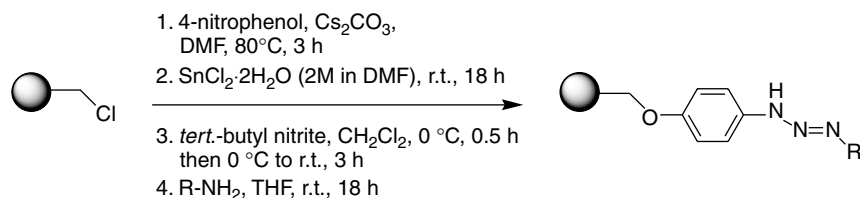
Scheme 2 Alkyltriazeno resins are prepared in four steps on Merrifield resin using primary alkylamines ( \text{R-NH}_2 ) in the last step.
